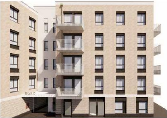
Brick Detailing to central piece amended. Horizontal textured brick detailing to pick up on ornate banded of conservation context buildings
